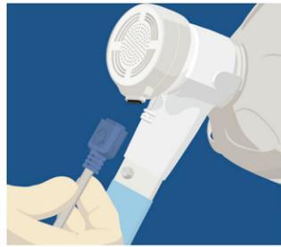
**STEP 2: ATTACH** magnetic side of ReddyPort Data Cable to microphone connector. The connector will only attach one way. If it is not connecting, simply switch its orientation.
