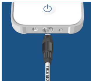
**STEP 3: PRESS** black end of data cable with text "this side up" facing the front of corresponding connector on controller until pins slide into place.
