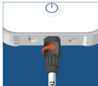
**STEP 4:** Once inserted completely, **ROTATE** locking collar on black end of data cable clockwise one quarter turn to secure and lock into place. If inserted correctly, you will hear it "click" and lock into place.
