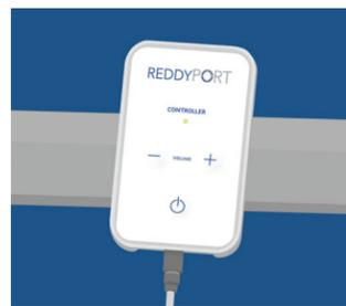
**STEP 3: PRESS** the power button on controller. The green LED light will illuminate. Adjust voice level utilizing up and down buttons on controller until the patient's voice can be understood
