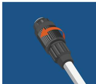
**STEP 2:** Before inserting data cable into bottom of controller, hold black end of data cable pointing away and turn rotating outer sleeve counterclockwise to open the locking mechanism.
